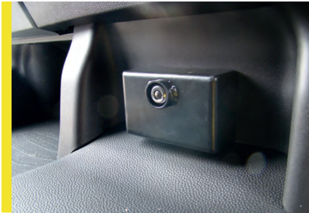
OBD lock protectors prevent unauthorised use of the port
