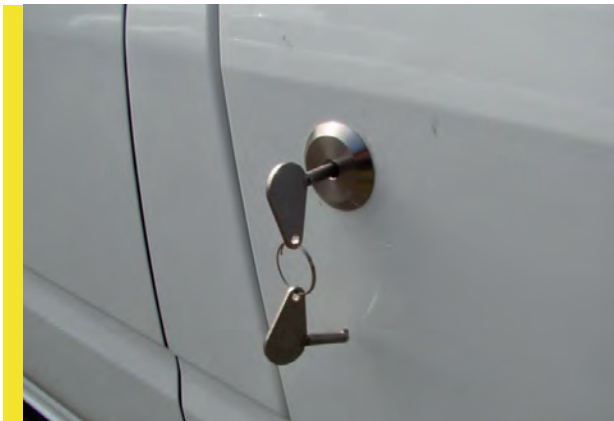
Installation of an anti pick replacement locking cylinder
