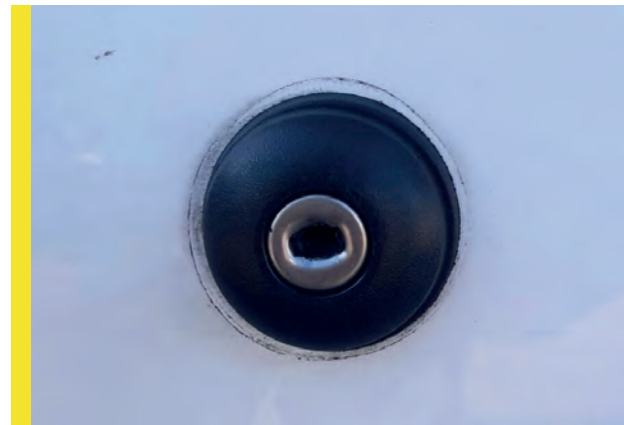
Typical example of an OE locking cylinder that has been attacked
