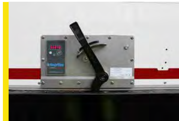
Electronic seals can help to improve load integrity, providing accountability and transparency of operations. Top to bottom (1): Maple Barndoor Freightlock, (2) Integration with telematics for real time door status and remote access control (3) Maple Integritas fitted to shutter door
