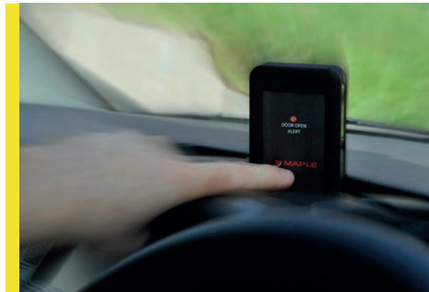
In-cab notification of curtain opening
